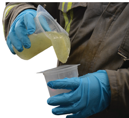
Fig. 8—The TriFrac-MLT crosslinked guar-based hydraulic-fracturing fluid developed by Trican and Emerald Surf Sciences.
