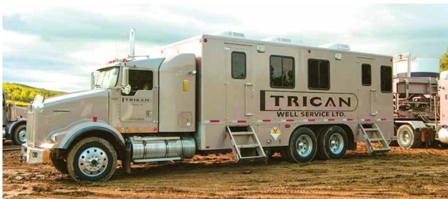
Fig. 3. Data acquisition and control van for hydraulic fracturing operations, complete with satellite communication equipment. Courtesy of Trican.
