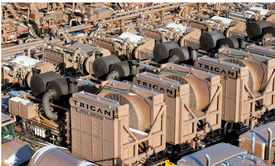
Fig. 4. Hydraulic fracturing pumps rigged in for multi-stage operations. Courtesy of Trican.
