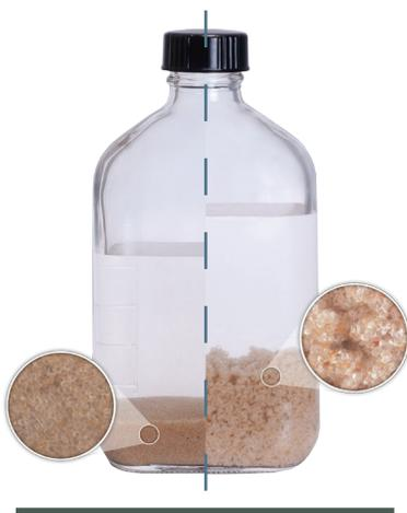
43g of settled proppant, following agitation. Conventional slick water slurry (left) and MVP Frac slurry (right).
